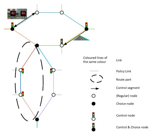
Figure 1 – Road network including all types of links, nodes and segments.
