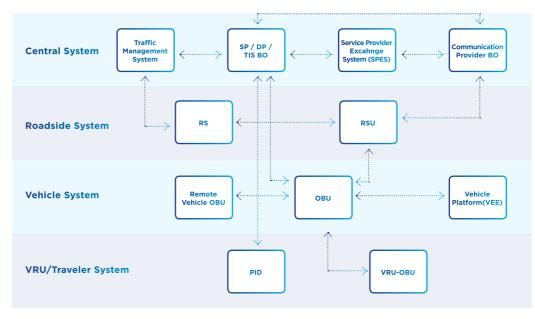
High-level functional architectural model for the C-MobILE applications
